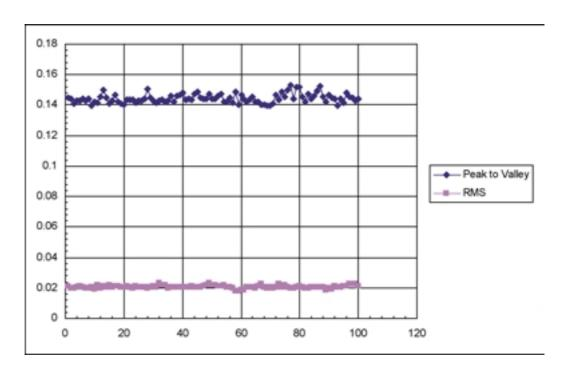
Variation over 100 measurements with Phase Shift software.
